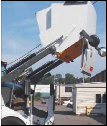
Front end flips up and over to dispose of waste.
