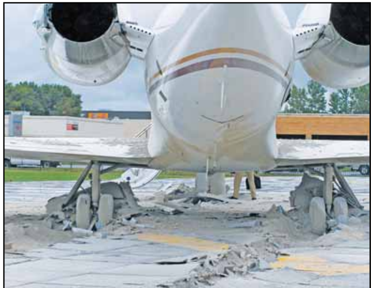
Damage done to the EMAS during the October 1, 2010 incident affected about 112 panels.
