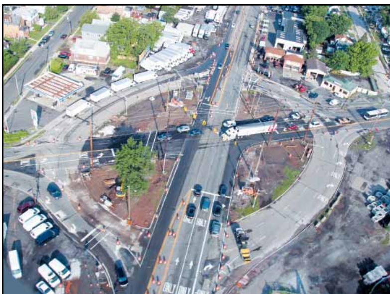
Little Ferry Circle Eliminated: Replaced with a 4-way Intersection, August 2014
