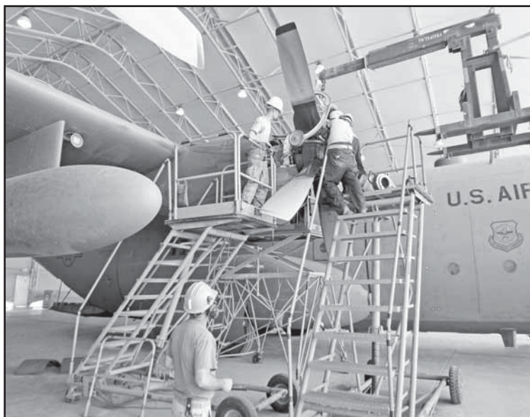
Navy Seabees assist the Air Force putting a new propeller on one of their C-130 aircraft using a 11K rough terrain forklift. "We have a great relationship with these folks."
