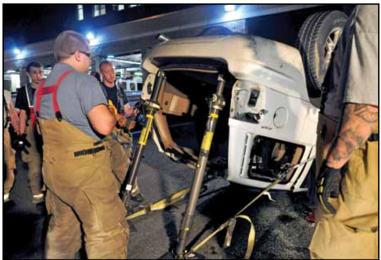
On October 10, 2018, the Carlstadt Fire Department performed heavy rescue training using Jaws of Life to cut up a vehicle. These hydraulic rescue tools are used by emergency rescue personnel to assist in vehicle extrication of crash victims. Jaws of Life tools include cutters, spreaders and rams. Photos by Dennis Kronymak Sr. ###
